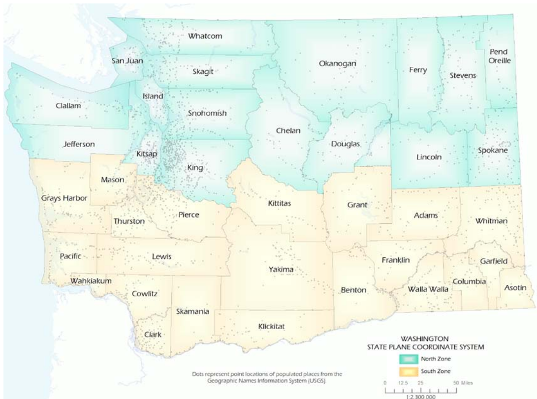
Figure 1 – Washington State Plane Zones with GNIS populated places, originally developed as part of an assignment for successful completion of a workshop concerning projections within the University of Redlands, MS GIS Program.
